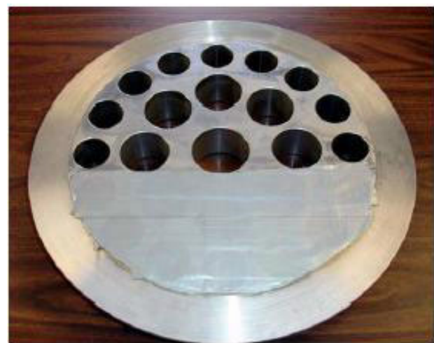
Figure 19 – 40% Blocked Flow Conditioner
