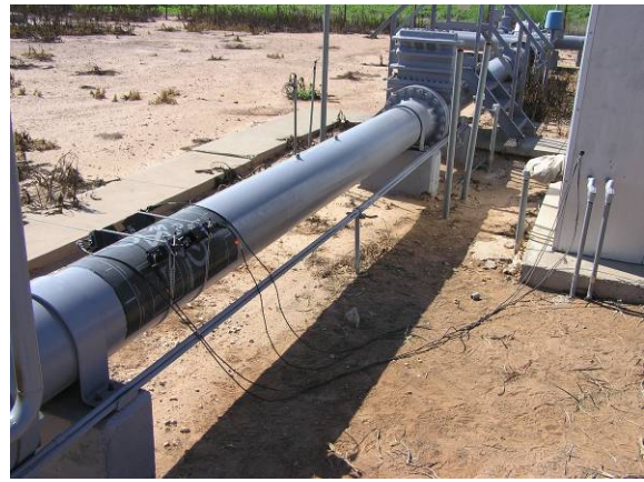
Figure I. Clamp-on Compared to Orifice Meter
